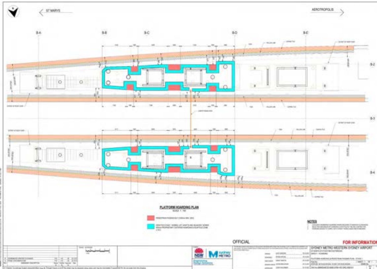
Figure 7: Preliminary platform hoarding plan for Stage 1 of the FSM works (Engineering Design Solutions 2022)
