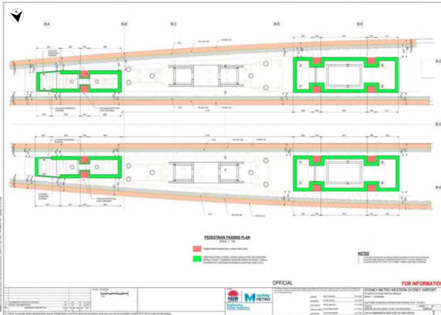
Figure 8: Preliminary platform hoarding plan for Stage 2 of the FSM works (Engineering Design Solutions 2022)
